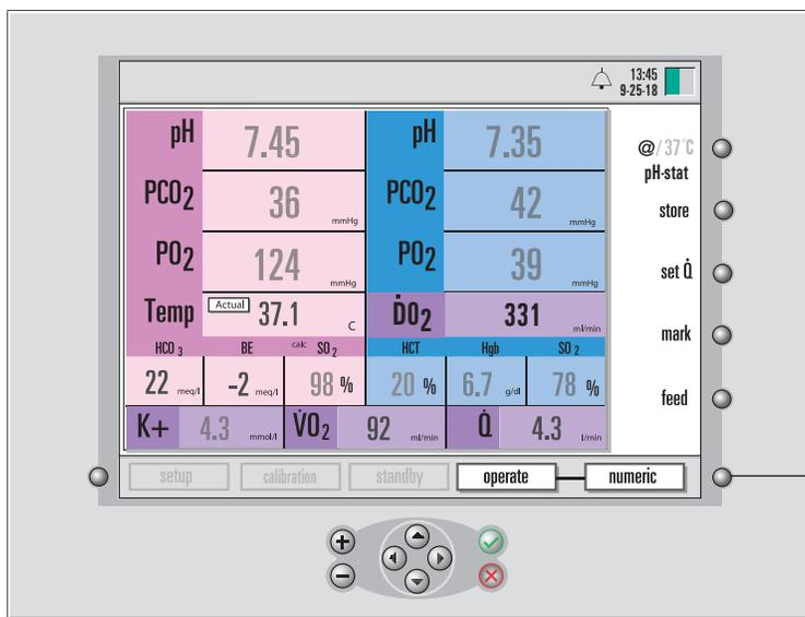
Press the operate mode toggle key to switch to a different display mode.
