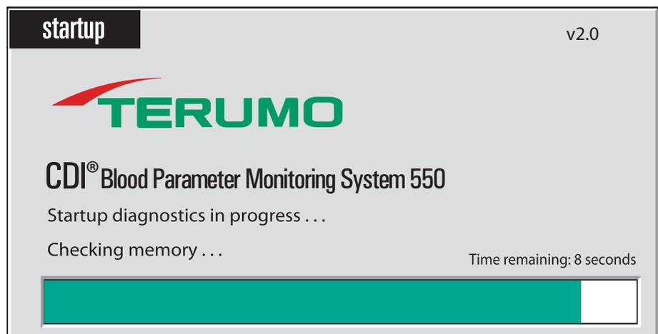
The system diagnostic testing takes about 40 seconds. During these diagnostics, the BPM self-test(s) and/or a CDI H/S Probe self-test are completed.
