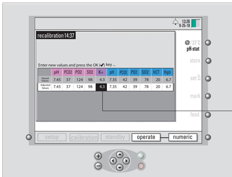
When the recalibration screen first opens, the potassium value is highlighted.
