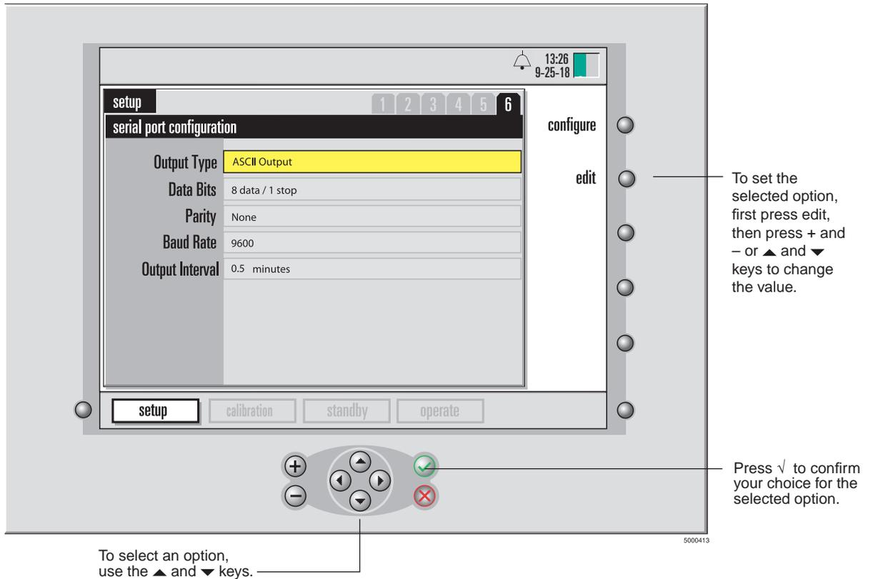
The following table lists the possible settings for the parameters on the serial port configuration screen.
