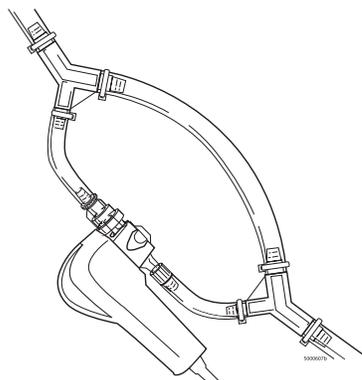
**Note:** If the Shunt Bypass Line has been placed in the bypass circuit and the CDI Shunt Sensor is not going to be used, one of the following steps should be taken:
