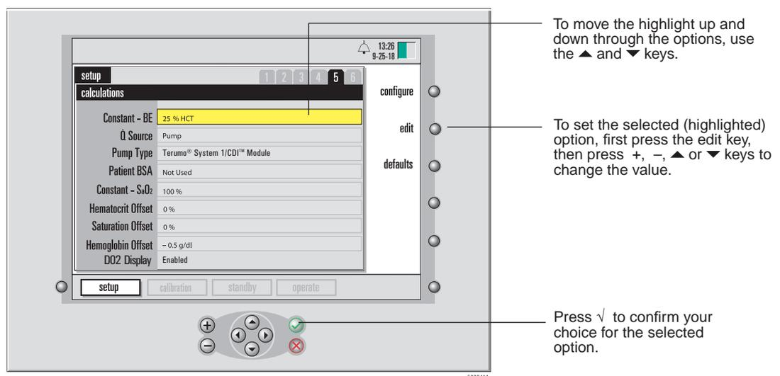
The following table explains the purpose and possible values for the settings on the calculations screen.
