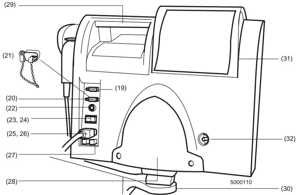
This figure shows the back panel of the monitor.
