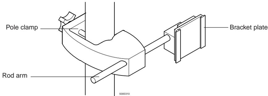
The cable-head bracket can be adjusted four ways:
