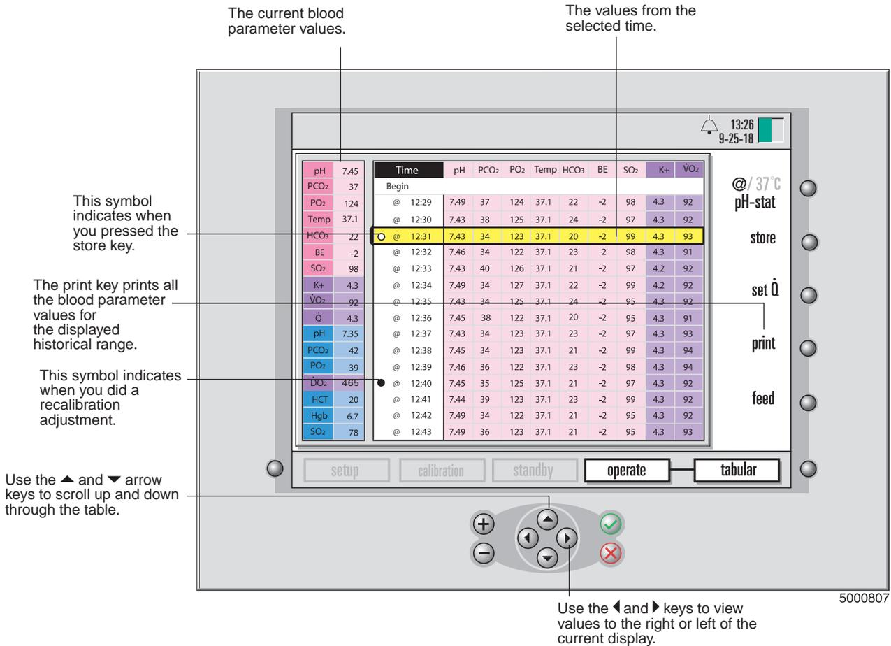
**Note:** Historical values are displayed in the original temperature mode (either actual or 37°C), regardless of the current temperature mode. The “@” symbol indicates the actual temperature mode. No symbol indicates 37° data.
