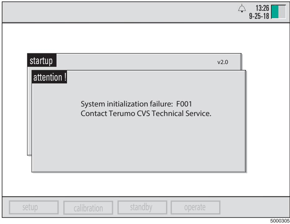
Errors that are recoverable will offer an option to continue — usually by pressing the √ (OK) key. Any consequences of continuing despite the error are noted in the error message. The message may recommend contacting Terumo Technical Service to resolve the error at a later time.
