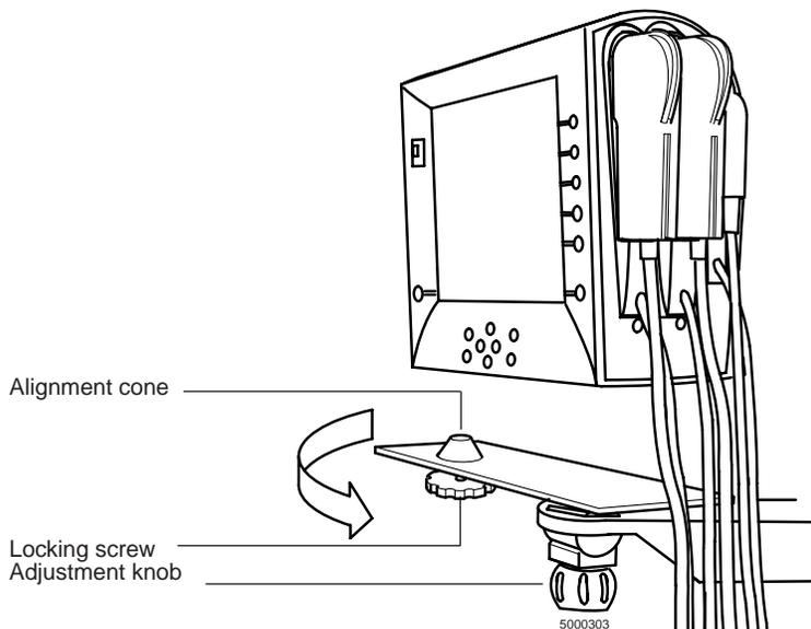
When you want to remove the monitor from the tray, you can loosen the locking screw until the monitor is no longer locked to the tray.
