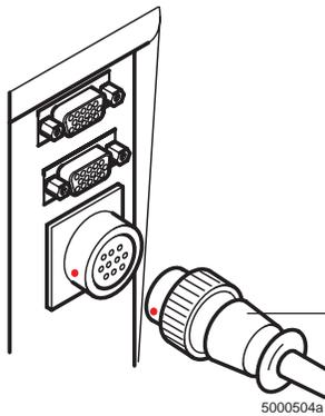
Connect the calibrator cable to the monitor by aligning the red dots on each of the connectors and pushing the calibrator cable connector onto the monitor connector.
