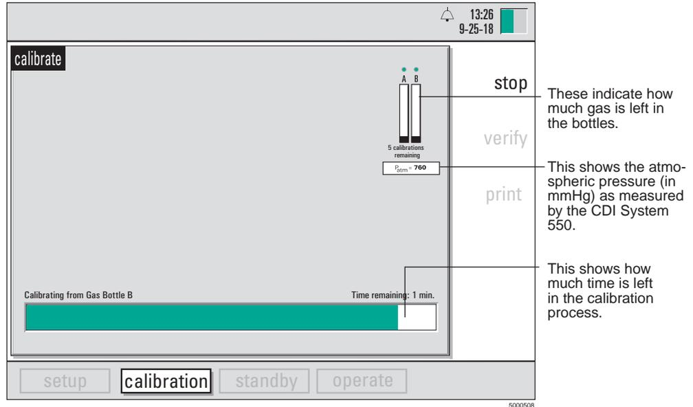
**Note:** The number of calibrations remaining, as displayed under the gas level indicators, reflects the approximate number of individual sensor calibrations left. If you are calibrating sensors for both arterial and venous monitoring, the count will decrease by two for each calibration procedure. A set of full gas bottles should provide enough gas for approximately 80 individual sensor calibrations.
